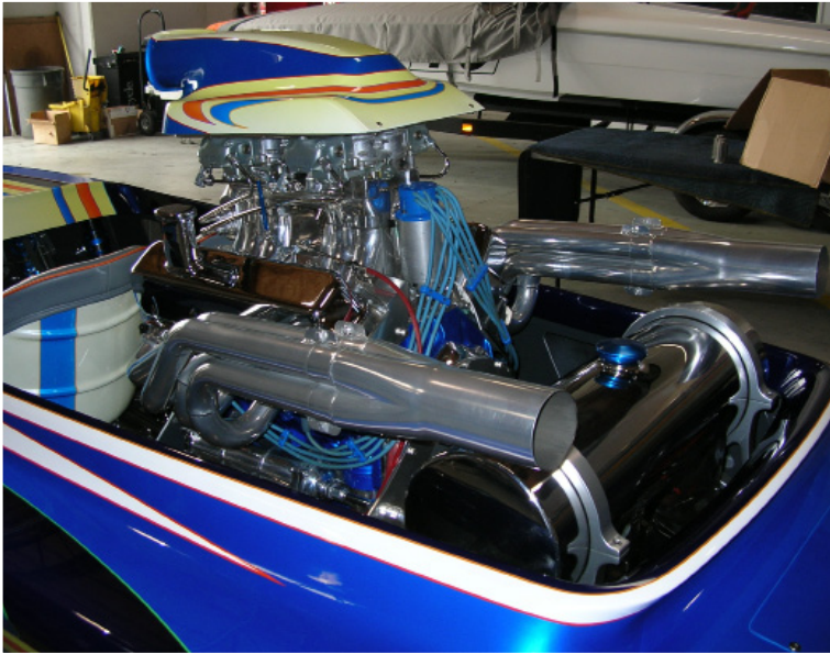
Ramirez took apart Kevin Kritzberger's Cole 22' Superhawk and added custom hardware, new dash and upholstery. It sports a modified Merc 800+ hp engine (below) and Bravo drive.
